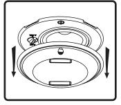
8. Remove paint mask unless painting is required. In that case, follow steps 9-12 when painting is complete.
